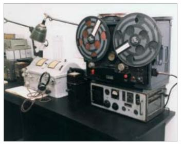
To receive and record news emitted by illegal transmitters, a short band receiver Spez.860 Bs. and tape recorder AEG, model Ton. S.b. were used.
