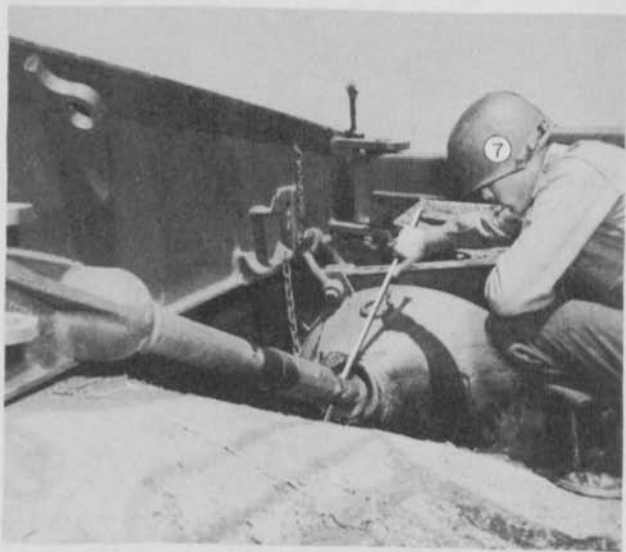
Figure 30. Adjusting an inside spade jack.
