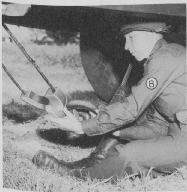
Figure 60. Attaching winch line to wagon jack line.
