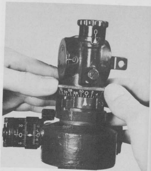
Figure 78. Slipping zero of the slipping azimuth scale to index on door.
