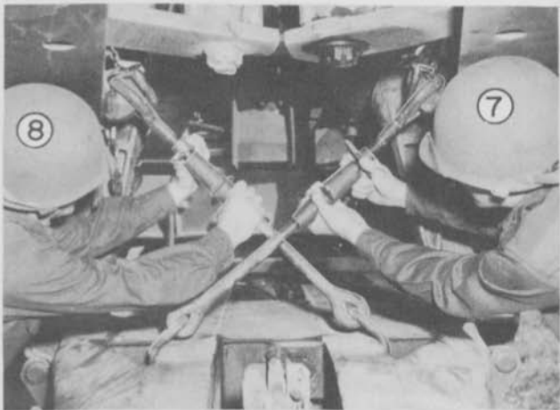
Figure 18. Removing trail cross braces.
