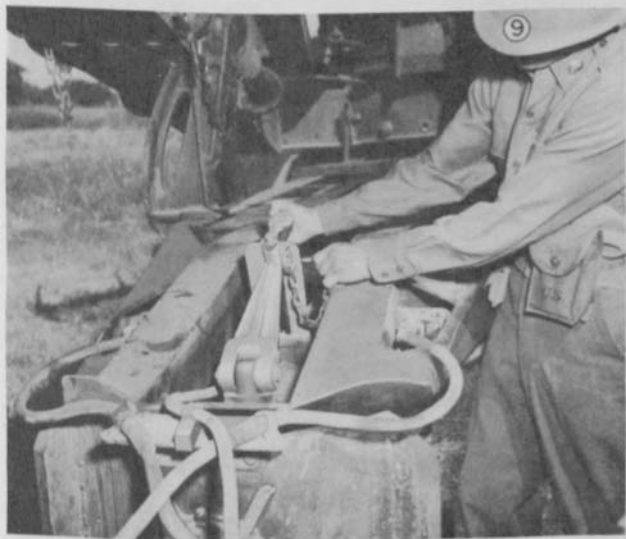
Figure 55. Removing lock lever pin from wagon lock lever.
