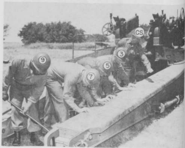
Figure 51. Spreading trails with assistance of winch cable.
