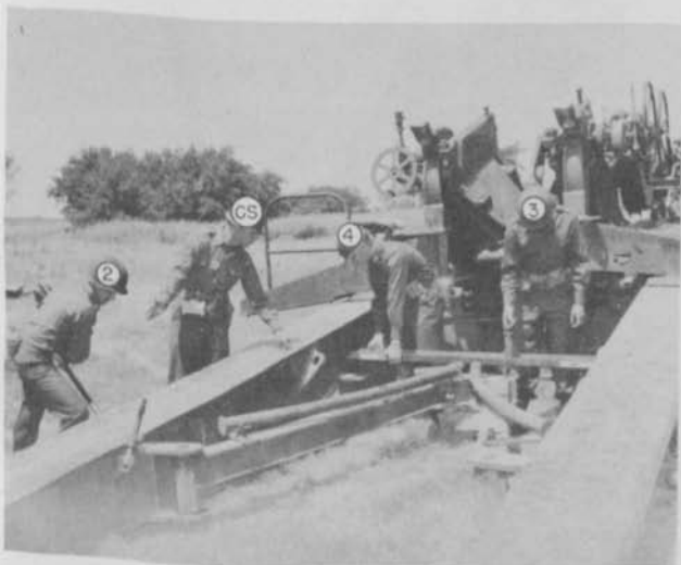
Figure 44. Emplacing trail spacer bar.
