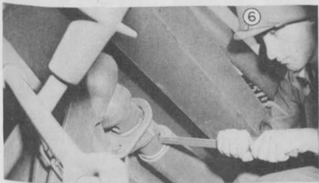
Figure 17. Loosening an inside spade jack in trail spade jack saddle.
