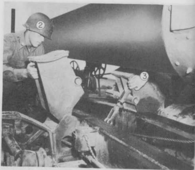
Figure 53. Removing tube support.
