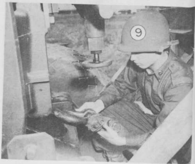
Figure 62. Attaching holding cable to front of carriage.
