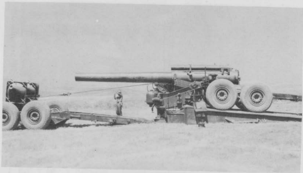
Figure 47. Winching tube forward to false cradle.
