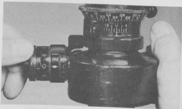
Figure 75. Loosening slipping micrometer scale locking nut.
