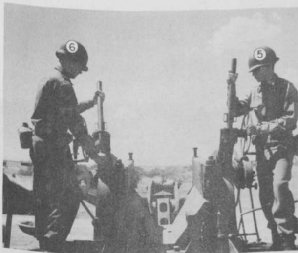
Figure 63. Attaching screw jacks to trunnion supports.
