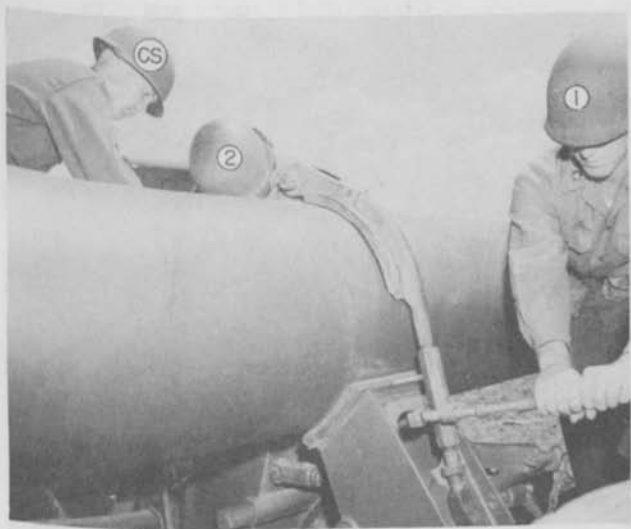
Figure 33. Removing the tube fastening strap.
