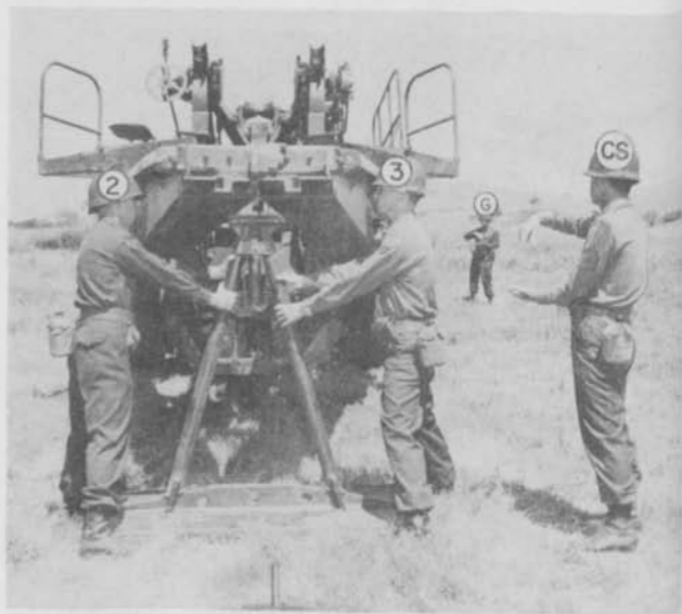
Figure 49. Emplacing trail support.
