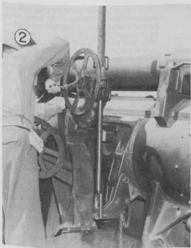
Figure 54. Operating screw jack to push keys down into keyway guides.
