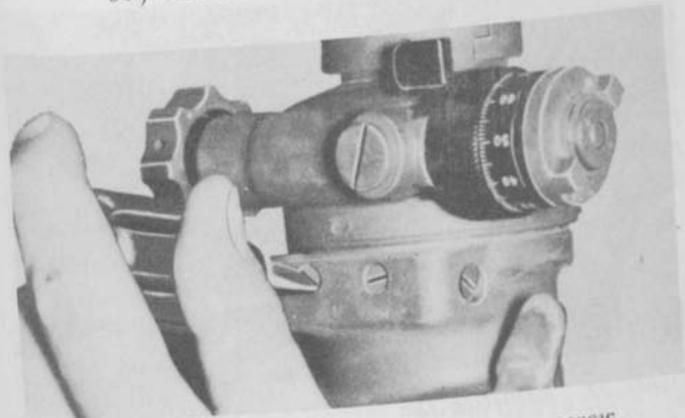
Figure 98. Loosening a tangent locking screw.
