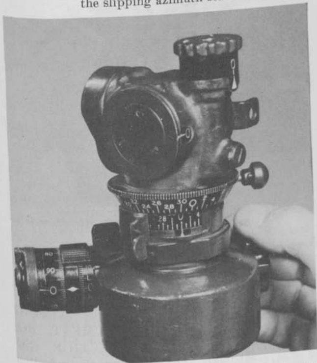
Figure 77. Turning the nonslipping azimuth scale to zero.
