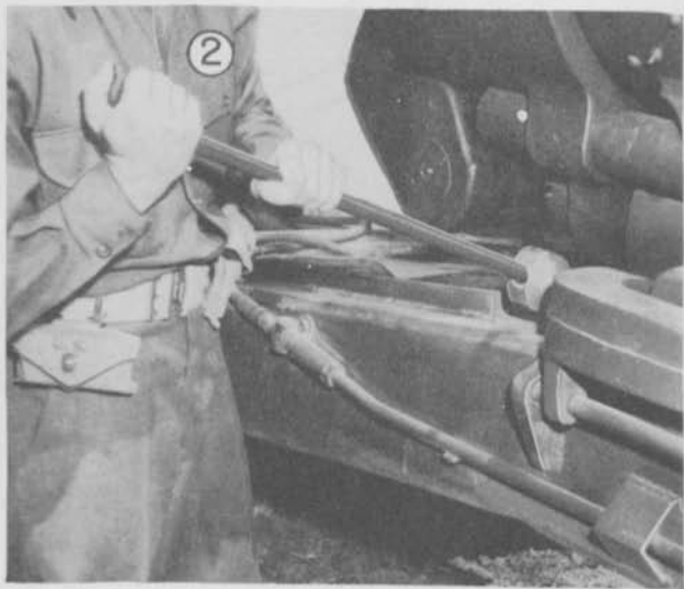
Figure 32. Unlocking the cradle traveling lock.
