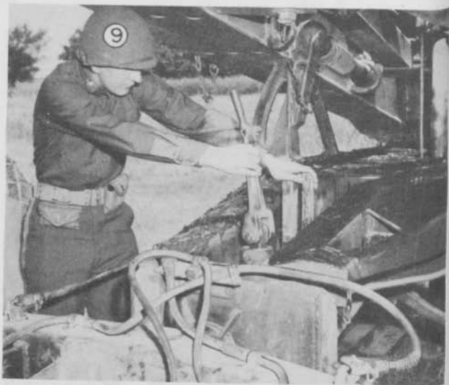
Figure 56. Removing wagon lock lever.
