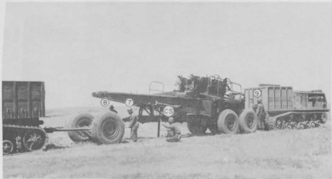
Figure 42. Removing front axle from carriage wagon.
