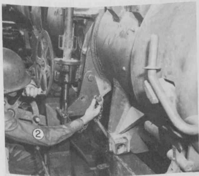
Figure 66. Securing jacking yoke prior to lifting tube to false cradle.
