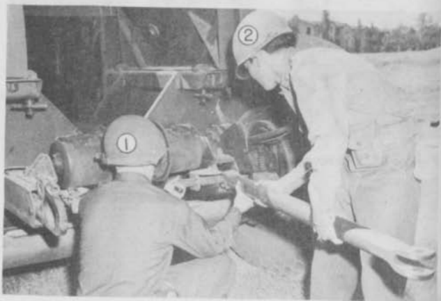
Figure 57. Assembling front drawbar on carriage transport wagon.
