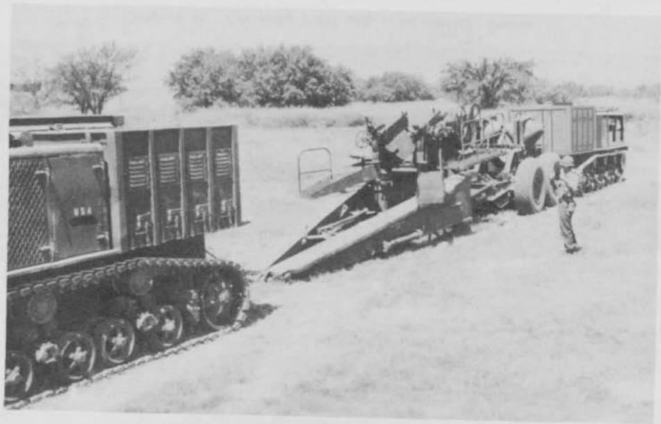
Figure 43. Removing carriage from transport wagon.
