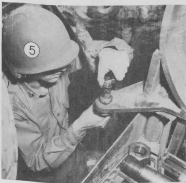
Figure 52. Fastening wagon attaching link to carriage.
