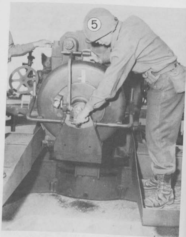
Figure 69. Inserting firing mechanism M1.
