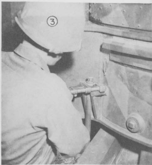
Figure 15. Loosening hold-down bolt of carriage.
