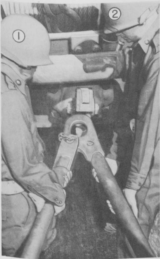
Figure 58. Attaching front drawbar to prime mover.
