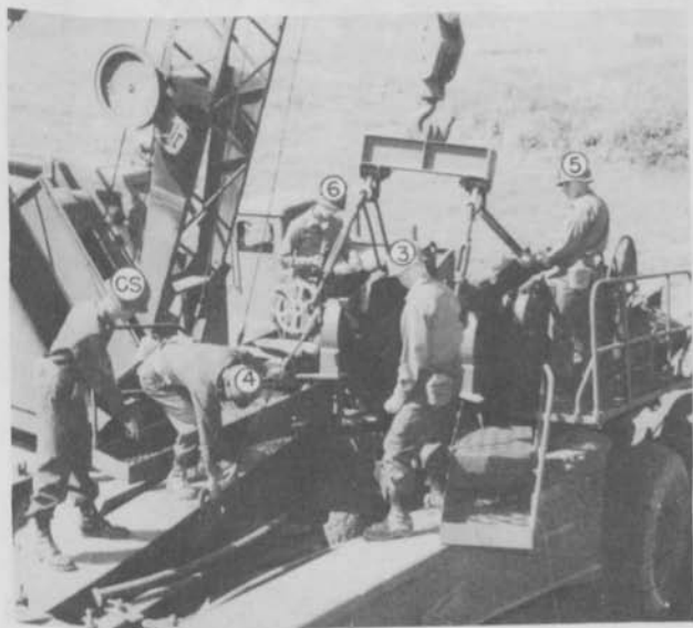
Figure 21. Attaching cable extensions.
