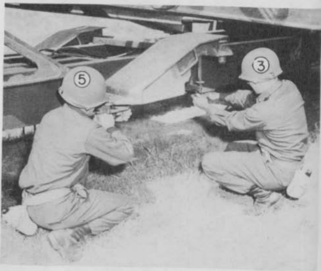
Figure 59. Removing wheel ramps.
