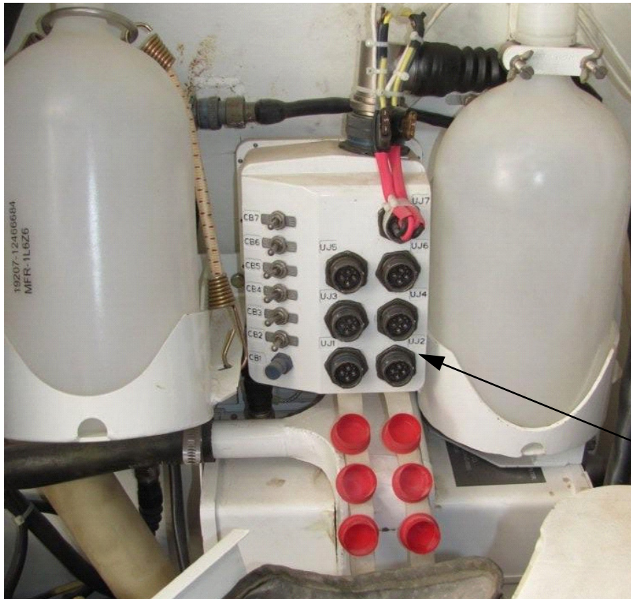
Figure 2-40 M1A2 with CROWS - Power Connection
