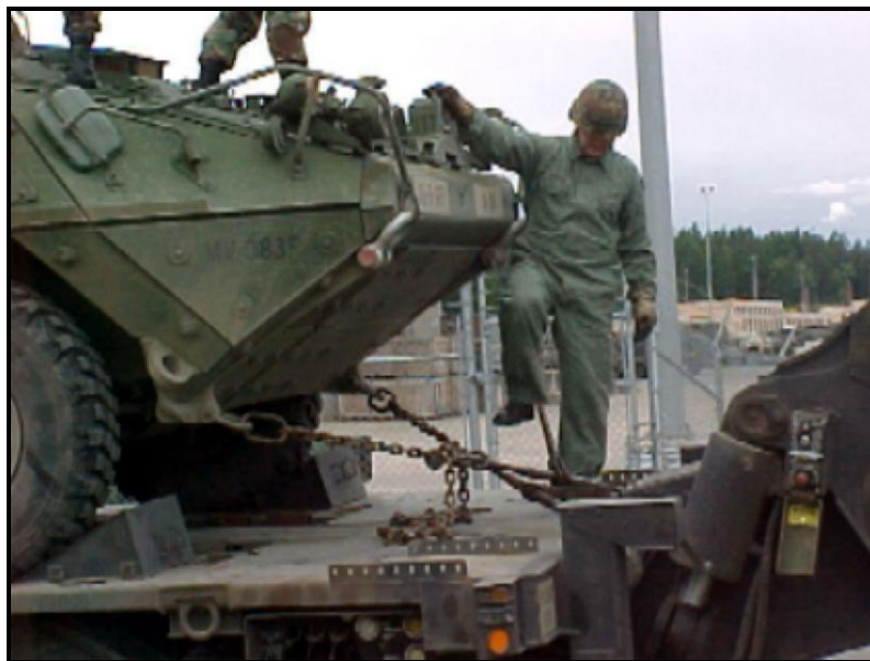
Figure A-4. Stryker secured on heavy equipment transporter (HET) front view.
