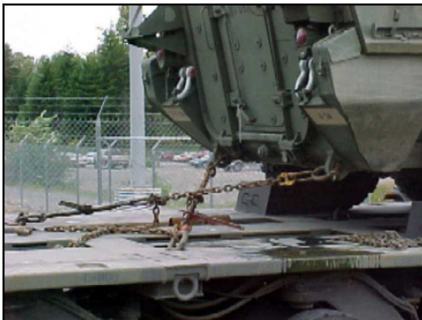
Figure A-5. Stryker secured on heavy equipment transporter (HET) rear view.
