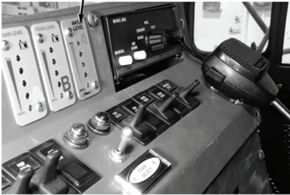
CAB WATER LEVEL GAUGE
