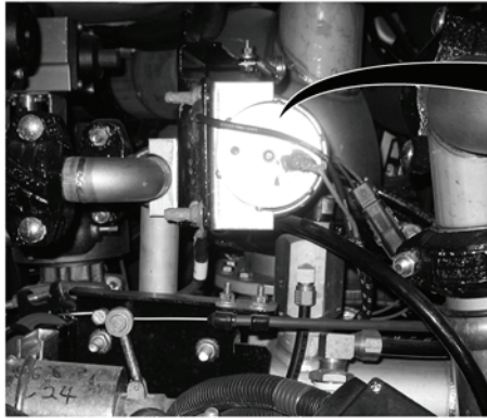
DRIVER MAIN INLET PRIMER VALVE TUBING TO DRIVER MAIN INLET VALVE ASSEMBLY
