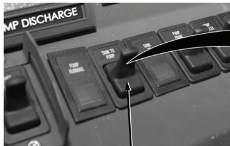
TANK TO PUMP SWITCH
