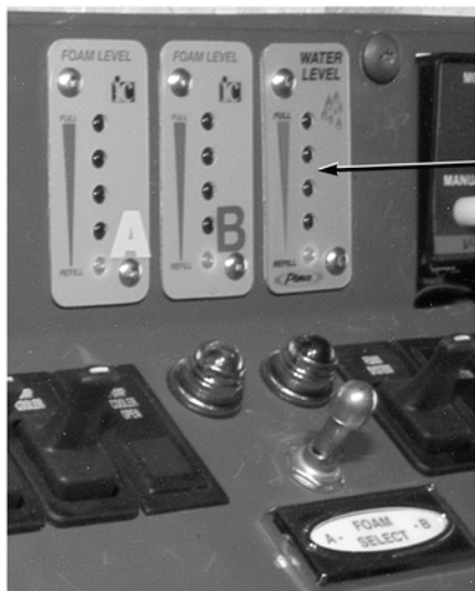
CAB WATER LEVEL GAUGE
