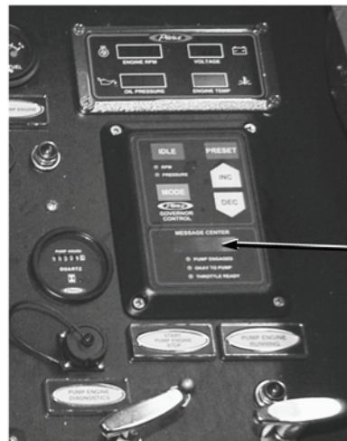
PRESSURE GOVERNOR CONTROL MESSAGE CENTER
