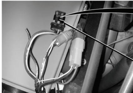
PUMP OPERATOR'S PANEL WIRE HARNESS EMR II INLINE FUSE HOLDER
