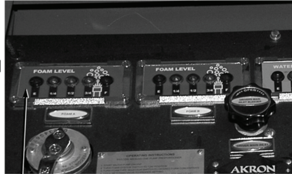
PUMP OPERATOR'S PANEL FOAM A LEVEL GAUGE
