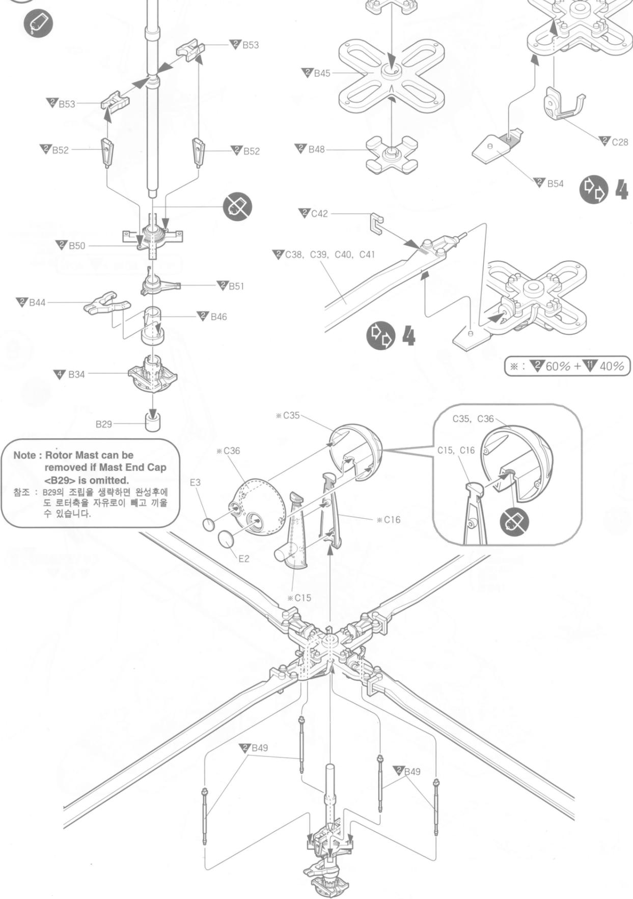
**Note : Rotor Mast can be removed if Mast End Cap <B29> is omitted.**
