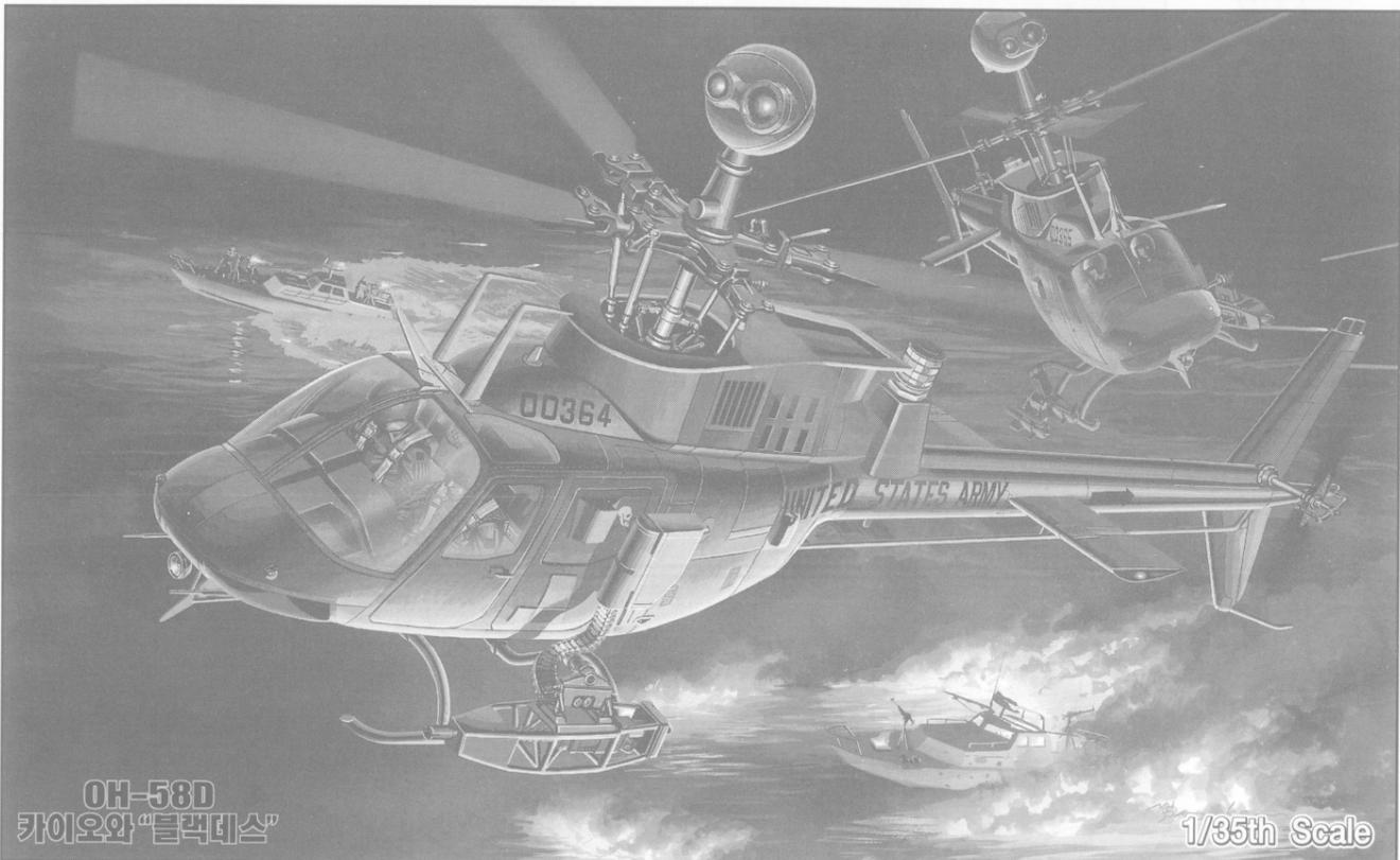
Bell's Model 206 was one of the top three machines in the U.S. Army's LOH(Light Observation Helicopter) competition in 1960. The Allison T63-A-5 turboshaft engine in the 206 yielded a cruising speed of 110 knots with a 400 pound payload. Afterward, the LOH program was on hold, but was opened again in 1967, and Bell's five-seat 206A Jet Ranger won that competition. The 206A was designated the OH-58A and deliveries to the U.S. Army began in May of 1969.
