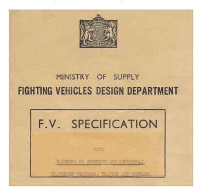
For AFVs (Armoured Fighting Vehicles) and MT (Mechanical Transport) vehicles the external bodywork was to be painted with an undercoat of Dark Battleship Grey BS Colour No. 32 (Air drying to Specification CS2390 or stoving to Specification CS2391). Followed by high gloss Deep Bronze Green BS Colour No. 24 (Air drying to Specification CS2392 or stoving to Specification CS2393 or heat resisting to Specification CS2394).
